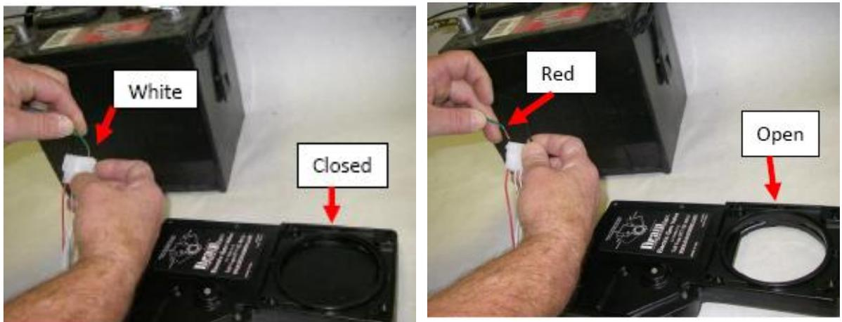
In the event the valve does not OPEN or CLOSE with the above procedure chances are good the valve has failed and needs to be replaced. If the valve works but is very sluggish (opens and closes but very slowly) the valve may need to be removed and cleaned. See Cleaning Procedure link Pg. 3
