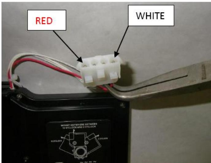
Using a 12 V DC battery or battery charger set on 12 V DC, put the White wire on the Positive terminal and the Red wire on the Negative terminal.
