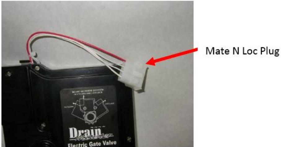
The 2 outer pins are the motor wires, a Red and a White wire, they come directly out of the back of the valve itself.
